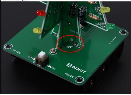
Step 20: Install 1pcs 3mm RGB LED at top. Pay attention to the direction of positive and negative pole.
