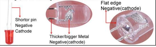
Step 4: Pay attention to the placement of the LED and then install 6pcs 3mm Red LED at D1-D6 on CTR-30A and bend the metal pins of the LED as shown for easy mounting. The square pad is the positive pole.
